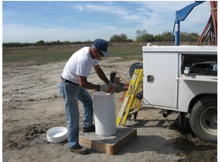
Staff member Jess Lopez draws water from a UWCD monitoring well along the coast.
