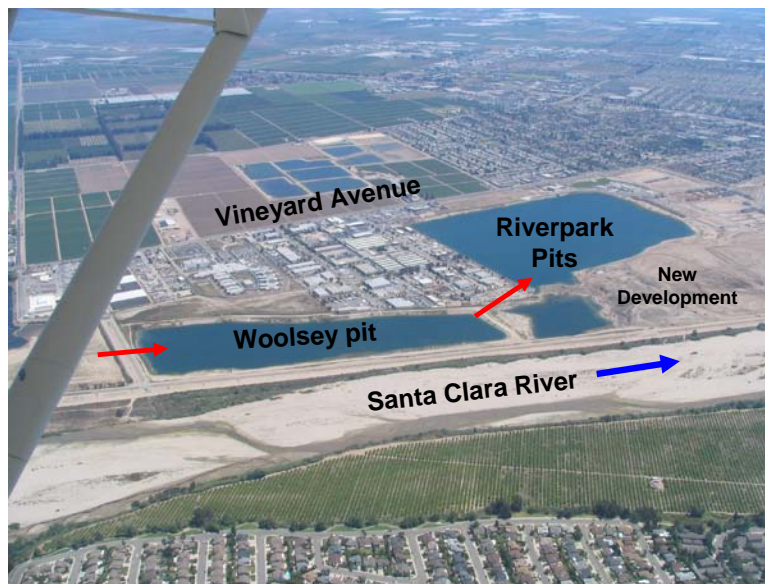
Figure 4. The Phase 1B Forebay Recharge Project would connect the Riverpark pits (including the Woolsey pit) into United's groundwater recharge system.
