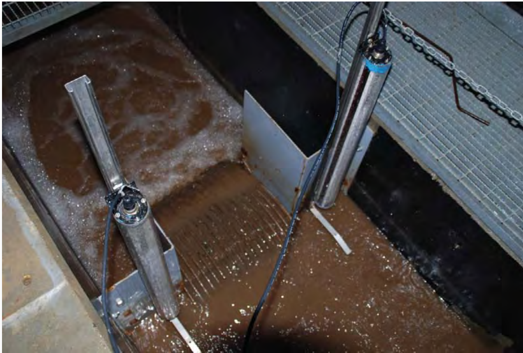
Photo 9 - Upstream Migration Monitoring Infrared Scanners
