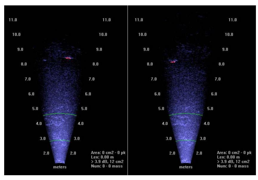
Figure 7. DIDSON images from April 28 (left) depicting a 426 mm fish moving upstream and May 13 (right), a 548 mm fish moving downstream. The body of the fish is indicated in red.
