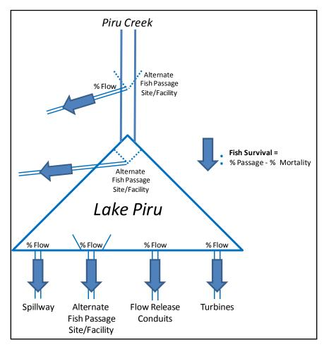
Figure 1. Conceptual schematic of downstream fish passage survival model under alternate fish passage facilities at Santa Felicia Dam and reservoir. Project survival calculated by totaling daily survival over the outmigration period during average, wet, and dry years.
