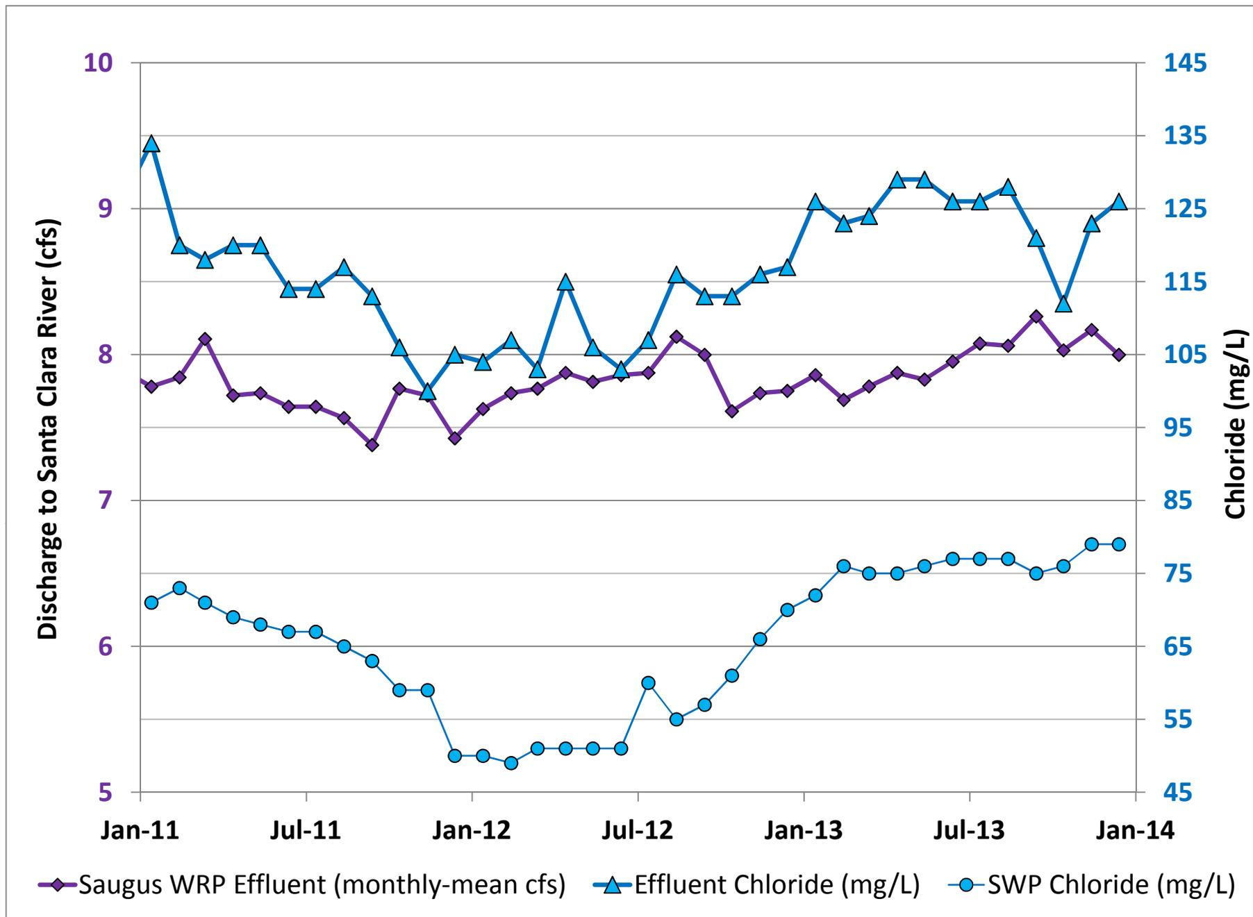
Figure 40. Saugus Wastewater Reclamation Plant effluent (NPDES) and chloride concentration discharge to Santa Clara River; State Water Project chloride concentration.
