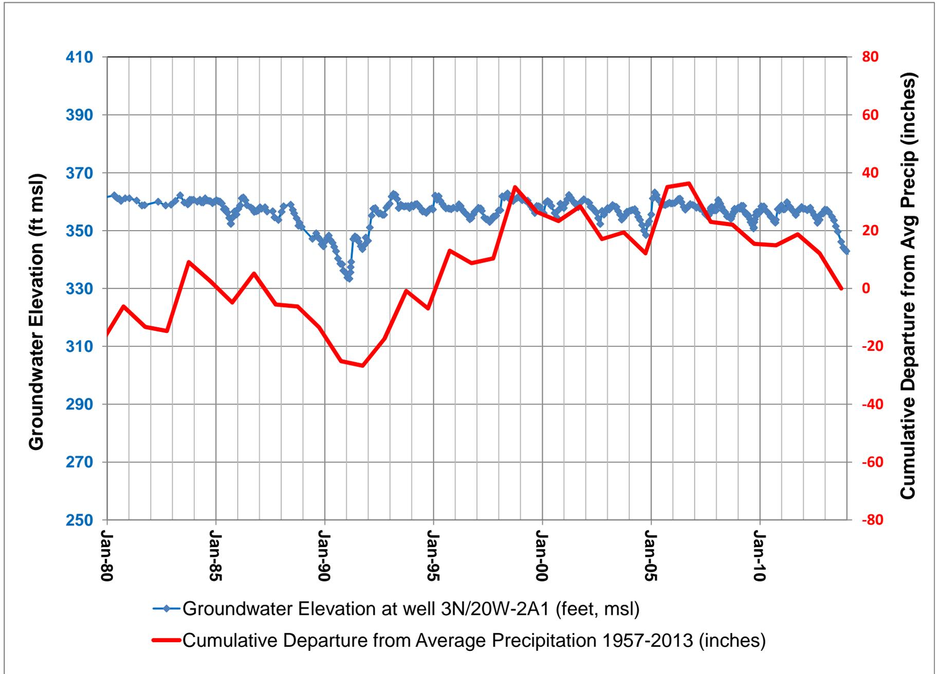
Figure 19. Groundwater elevations and cumulative departure from average precipitation for the Fillmore basin.
