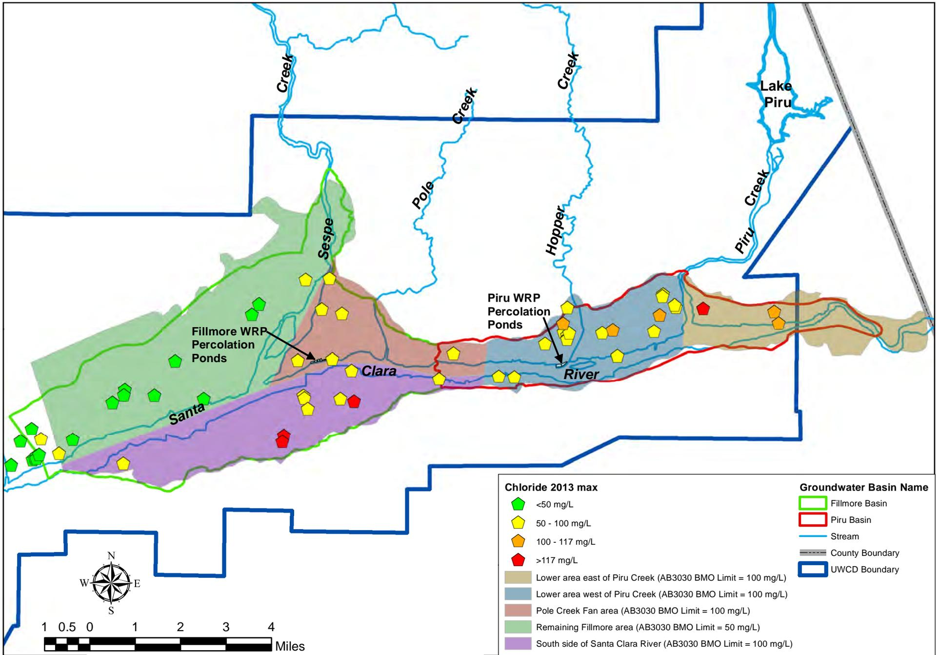
Figure 32. Chloride groundwater quality map of 2013 maximum concentrations (mg/L).
