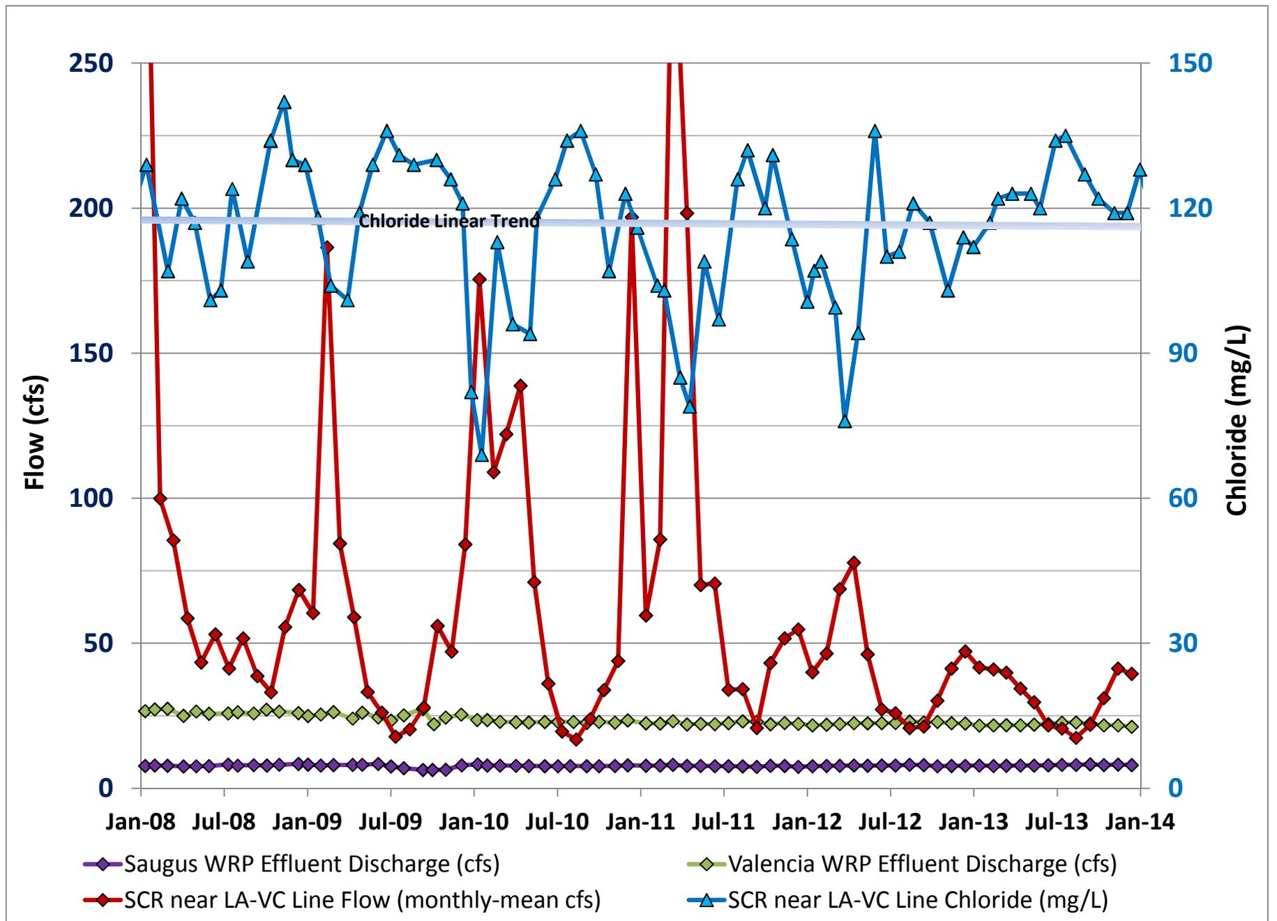
Figure 42. Saugus and Valencia WRPs effluent (NPDES); Santa Clara River flow and chloride concentration near the Ventura/Los Angeles County Line.
