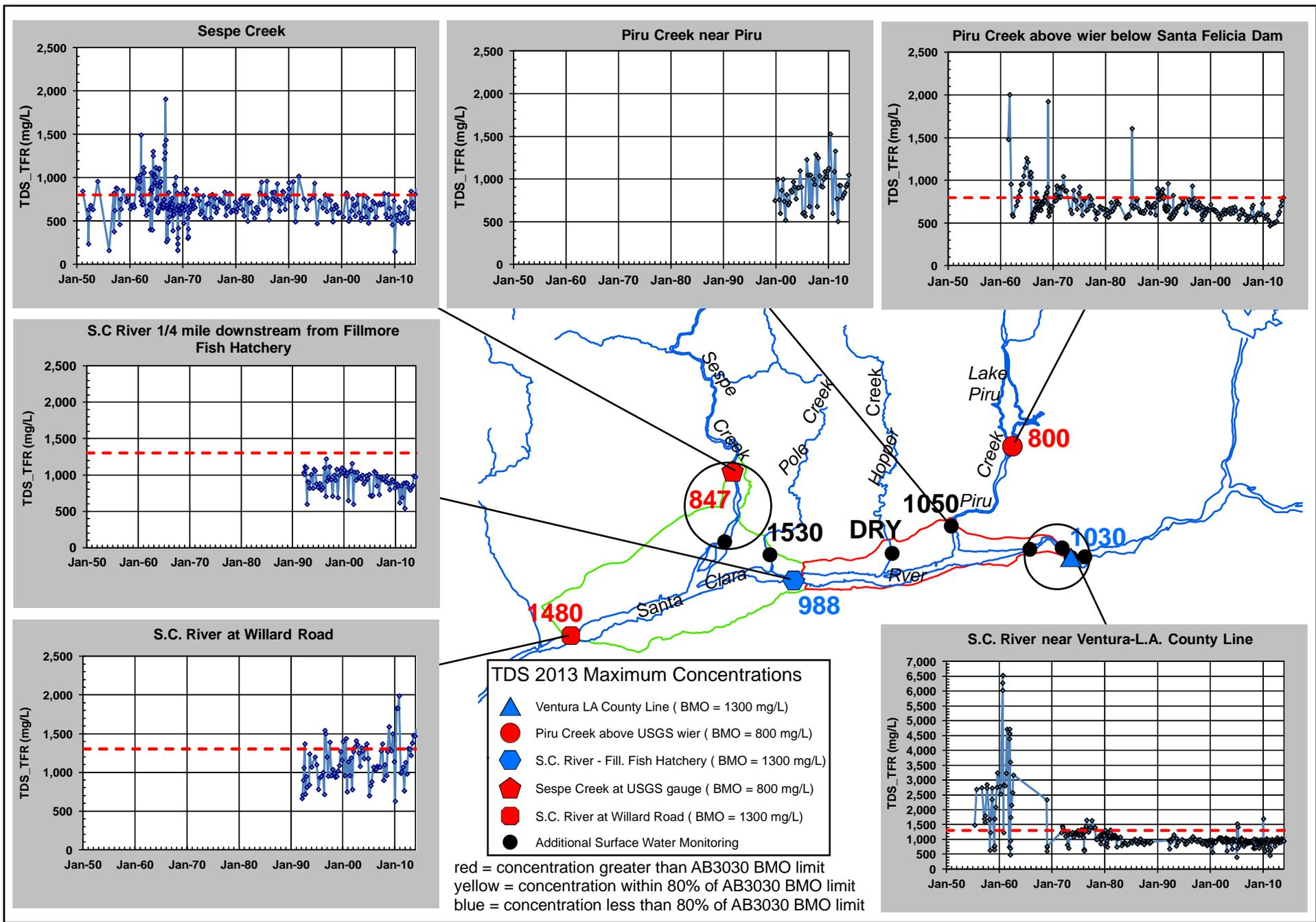
Figure 25. TDS surface water quality time series graphs with map of 2013 maximum concentrations (mg/L); dashed red line is AB 3030 BMO.
