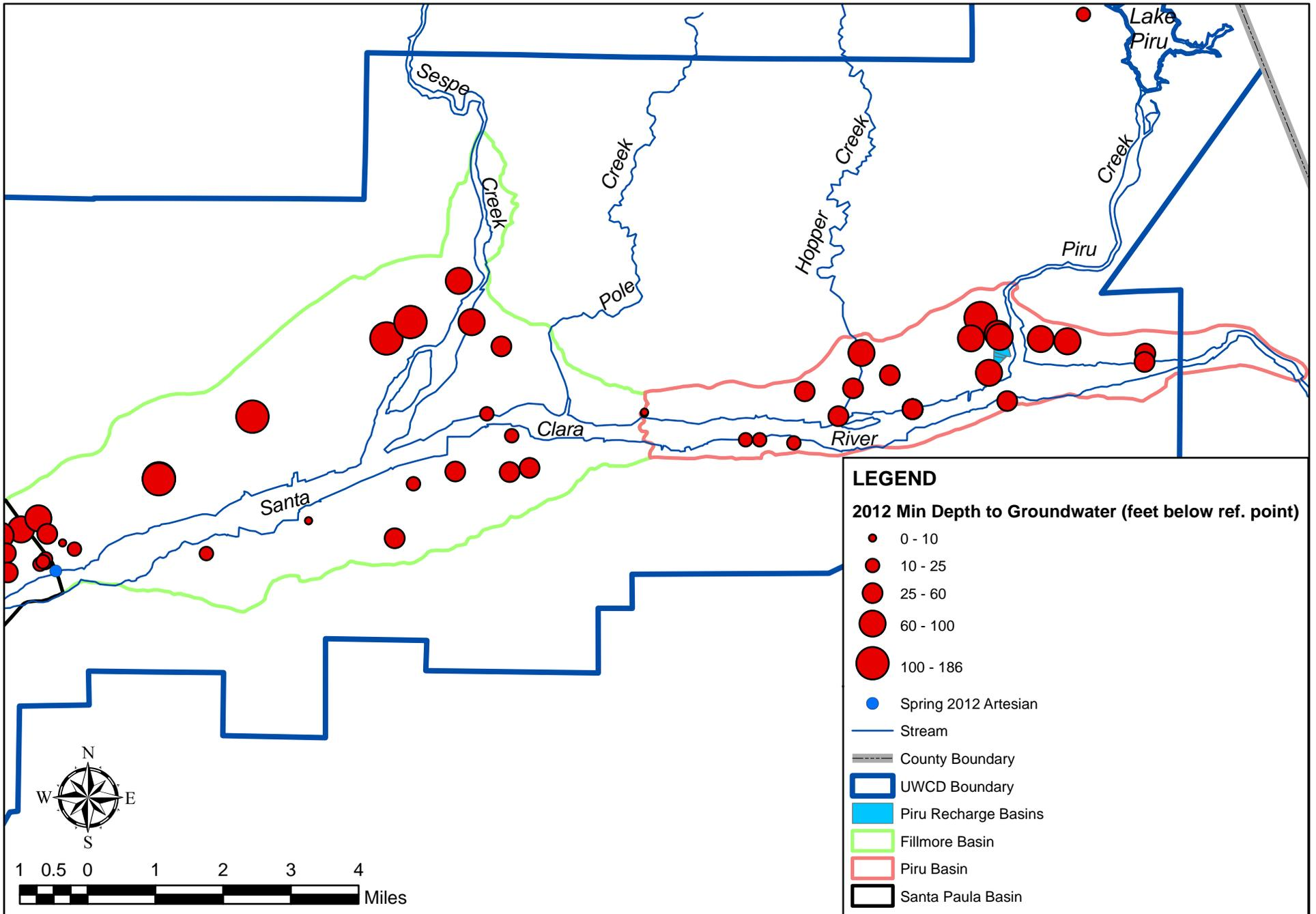
Figure 22. Spring 2012 depth to groundwater.
