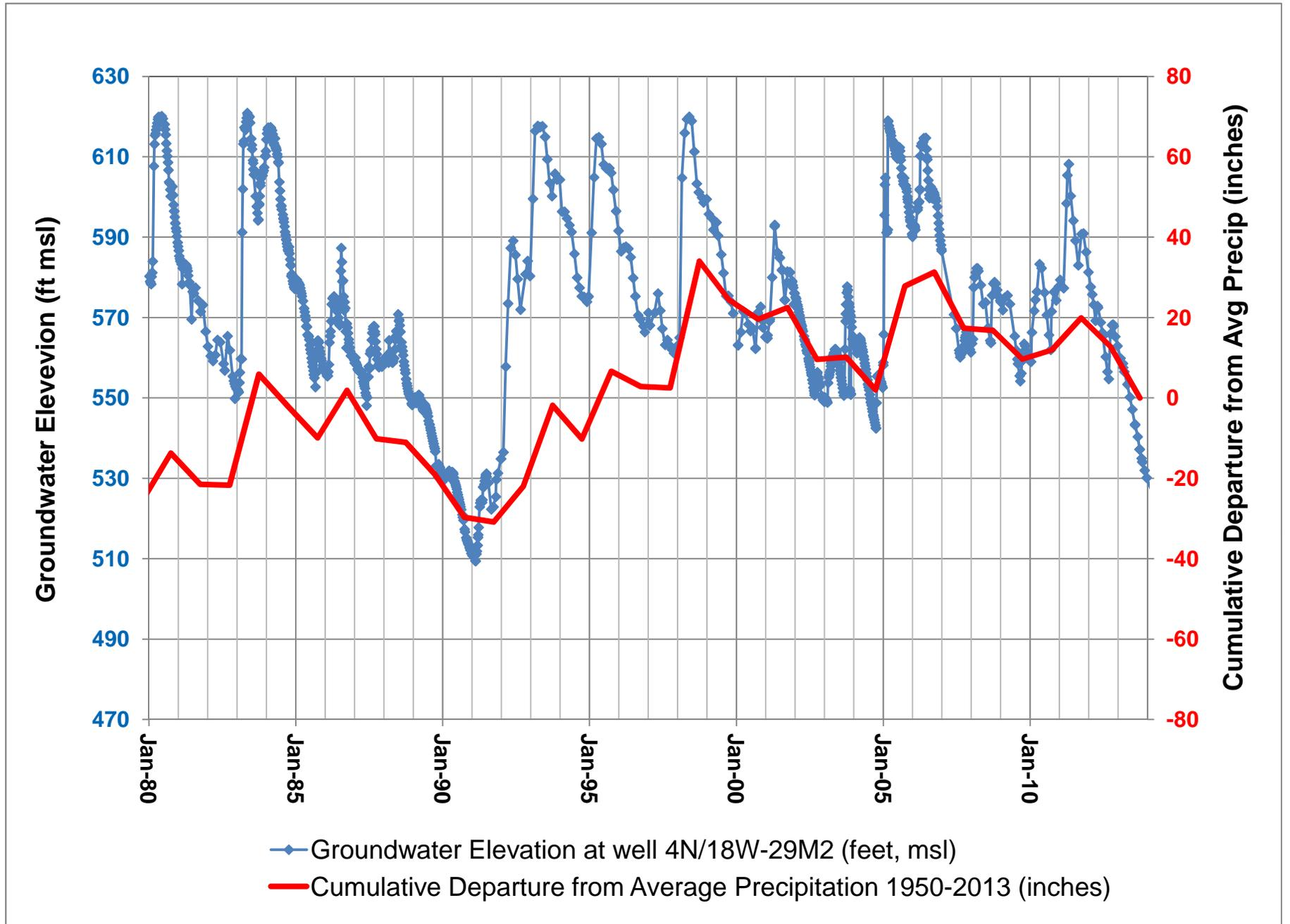
Figure 18. Groundwater elevations and cumulative departure from average precipitation for the Piru basin.
