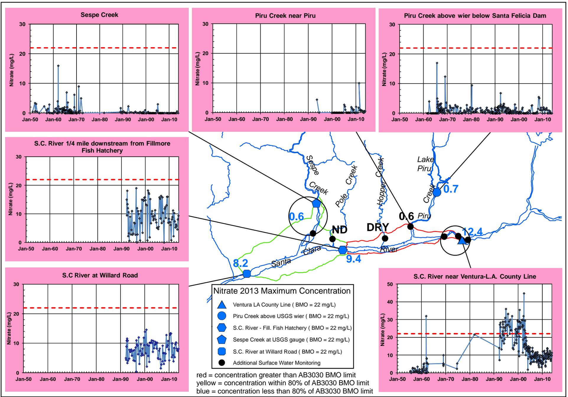
Figure 28. Nitrate surface water quality time series graphs with map of 2013 maximum concentrations (mg/L as NO<sub>3</sub>); dashed red line on graphs is AB 3030 BMO.
