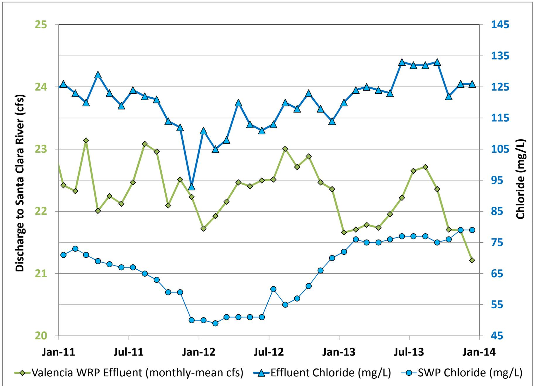
Figure 41. Valencia Wastewater Reclamation Plant effluent (NPDES) and chloride concentration discharge to Santa Clara River; State Water Project chloride concentration.
