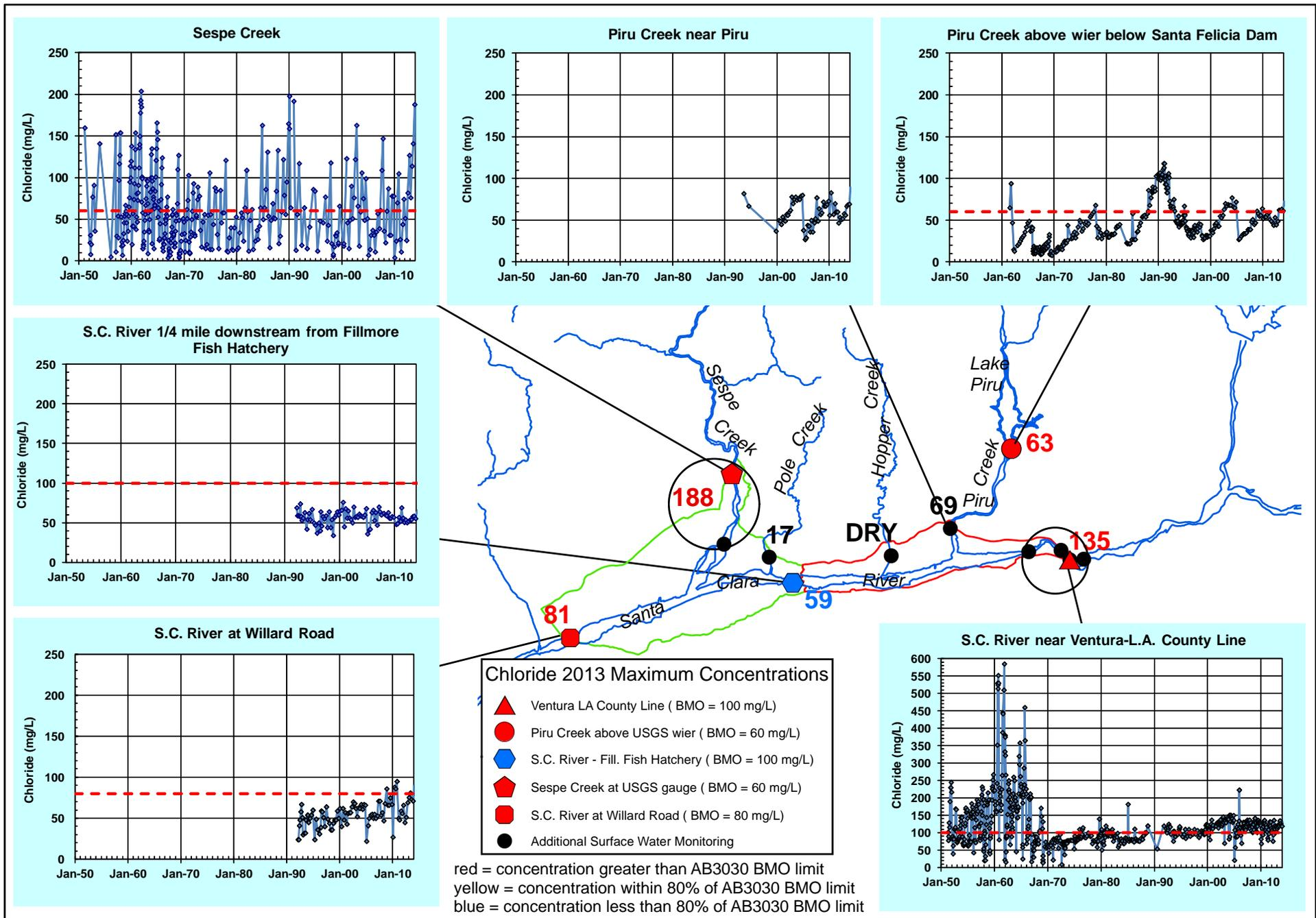
Figure 27. Chloride surface water quality time series graphs with map of 2013 maximum concentrations (mg/L); dashed red line is AB 3030 BMO.
