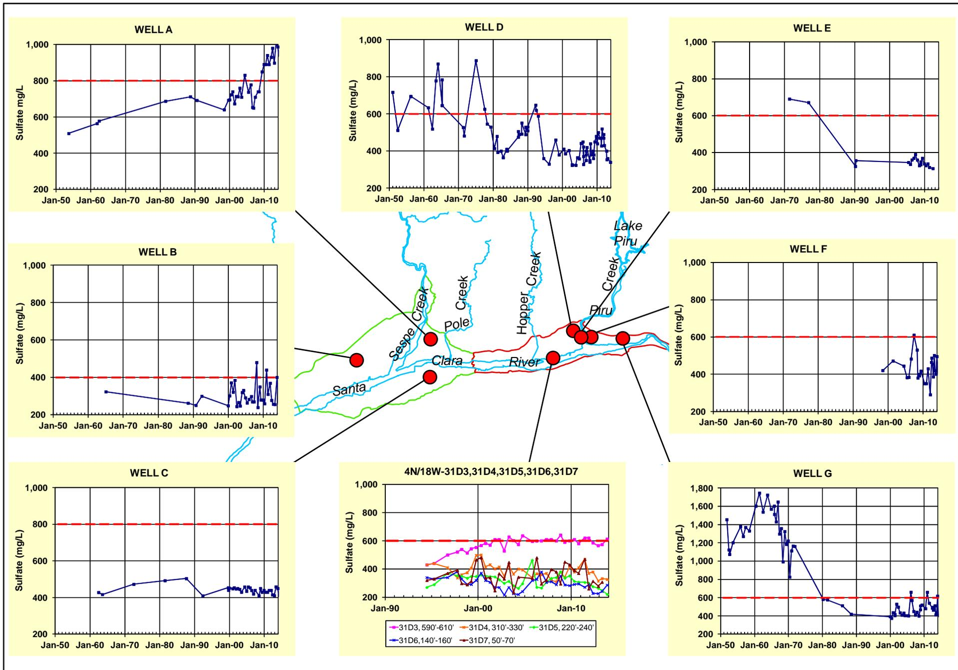
Figure 36. Sulfate groundwater quality time series graphs (mg/L); dashed red line is AB 3030 BMO.
