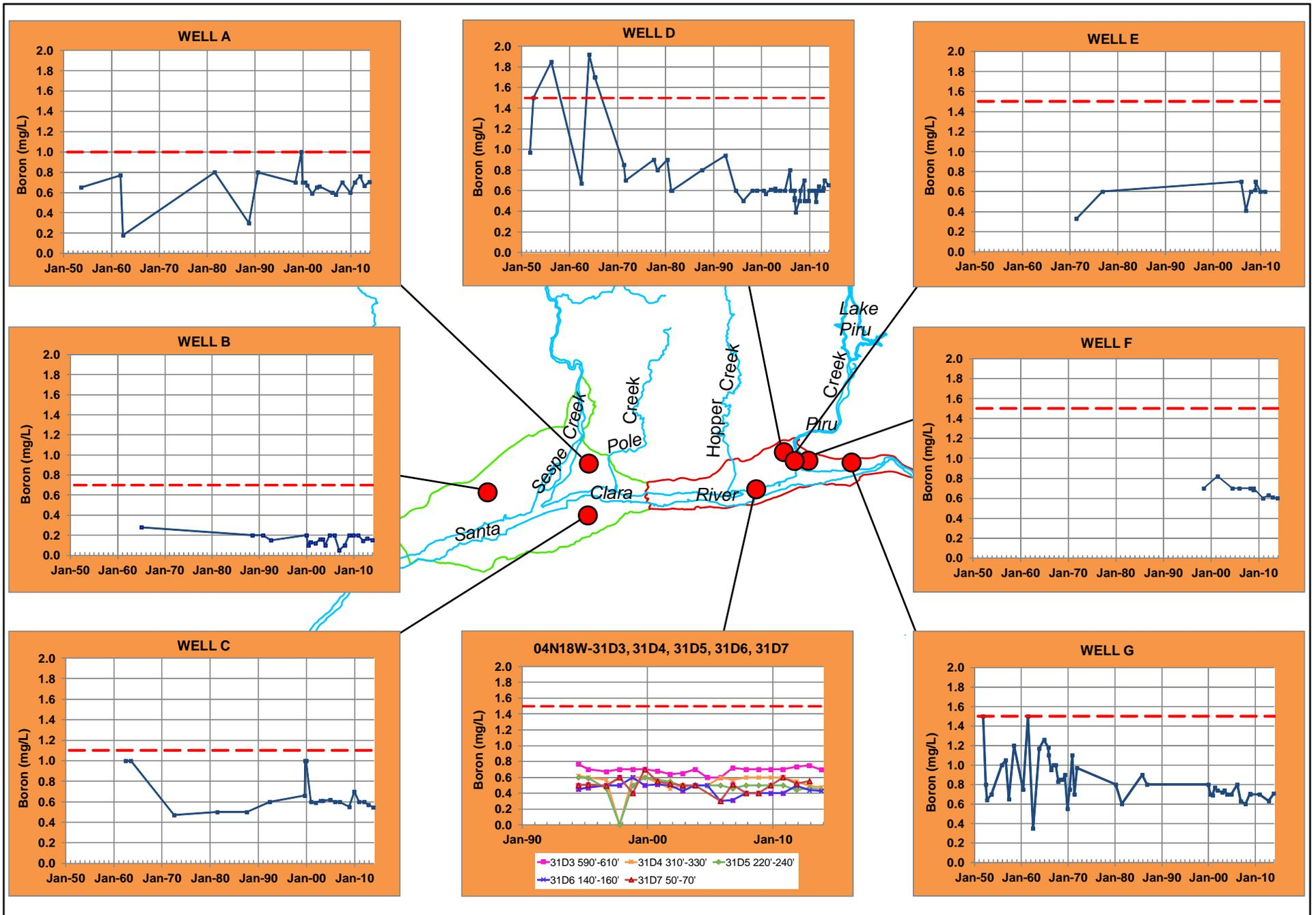
Figure 39. Boron groundwater quality time series graphs (mg/L); dashed red line is AB 3030 BMO.
