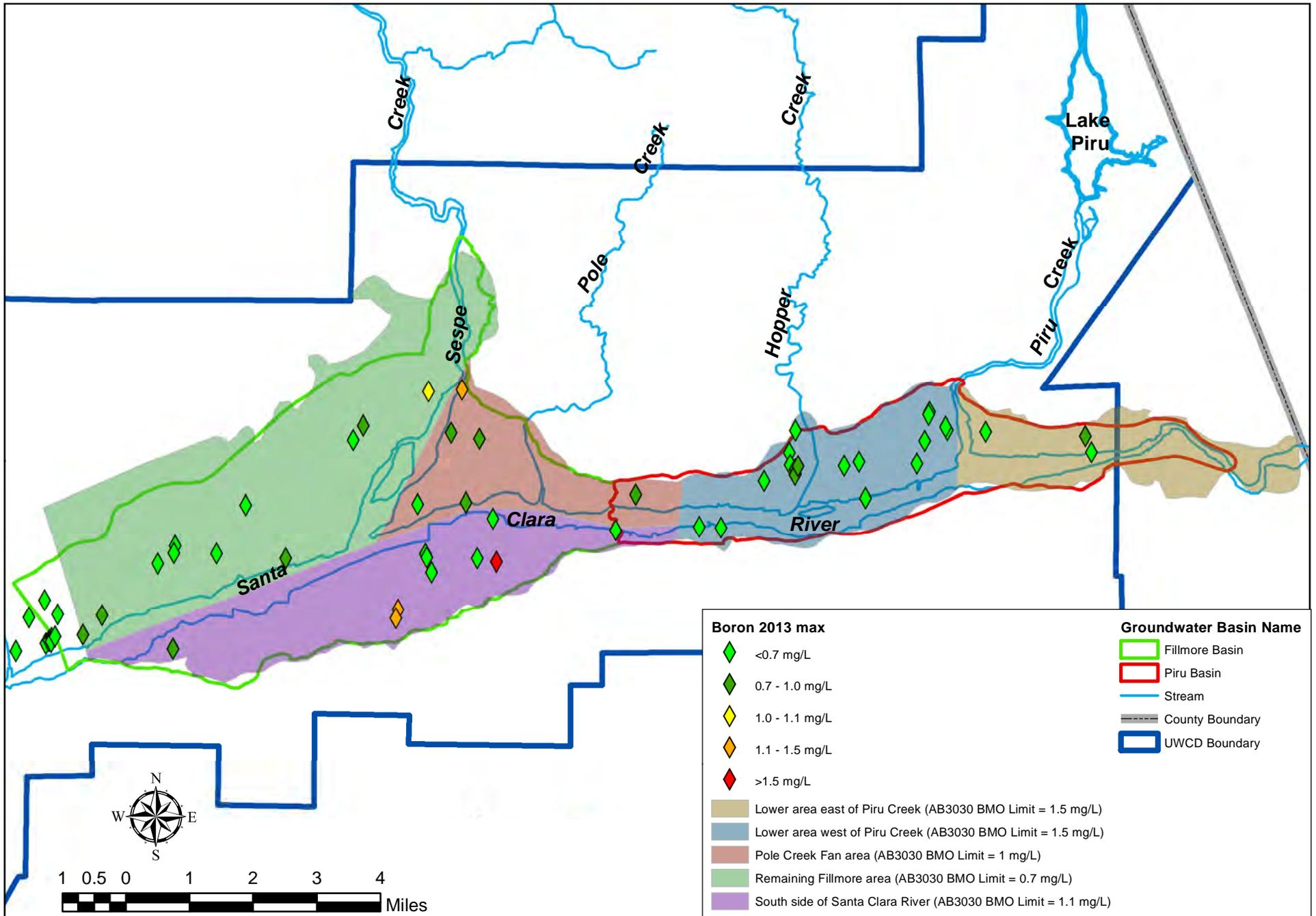
Figure 34. Boron groundwater quality map of 2013 maximum concentrations (mg/L).
