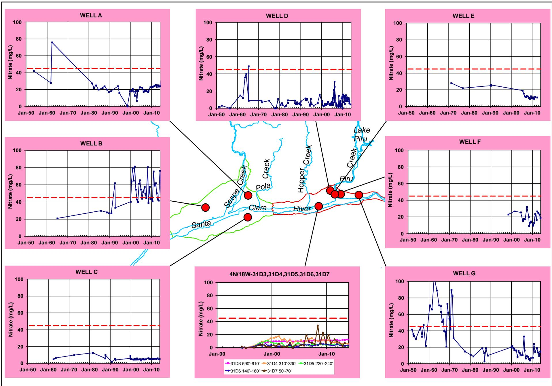
Figure 38. Nitrate groundwater quality time series graphs (mg/L as NO<sub>3</sub>); dashed red line is AB 3030 BMO.
