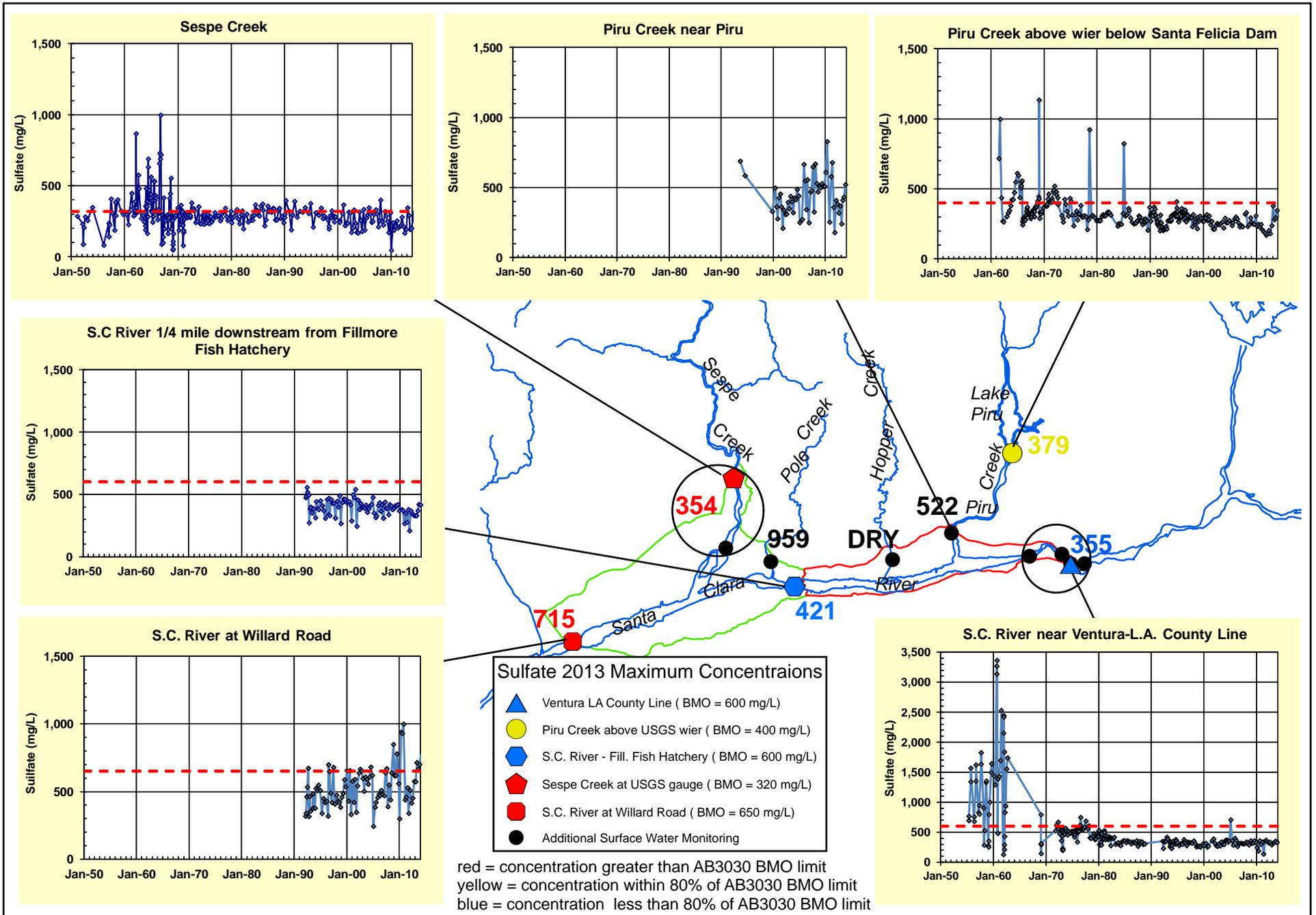
Figure 26. Sulfate surface water quality time series graphs with 2013 maximum concentrations (mg/L); dashed red line is AB 3030 BMO.
