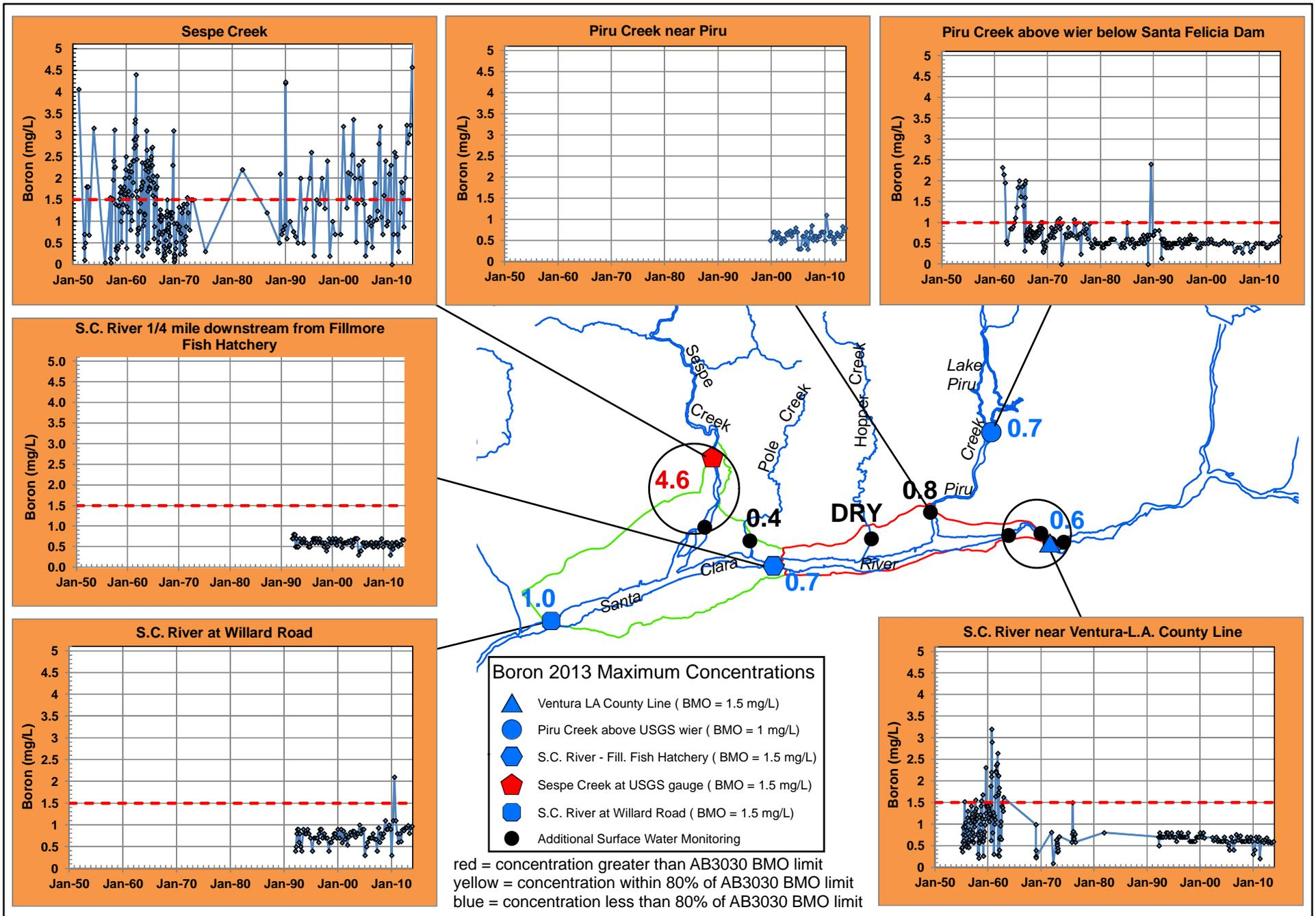
Figure 29. Boron surface water quality time series graphs with map of 2013 maximum concentrations (mg/L); dashed red line is AB 3030 BMO.
