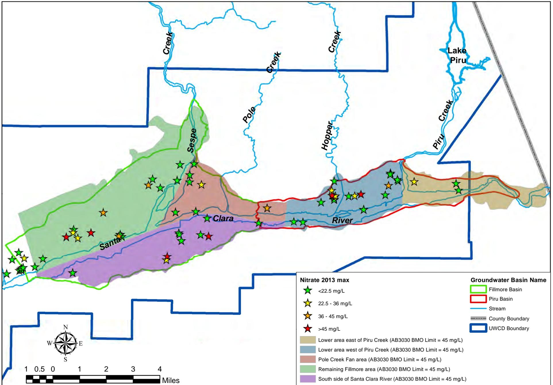
Figure 33. Nitrate groundwater quality map of 2013 maximum concentrations (mg/L as NO<sub>3</sub>).
