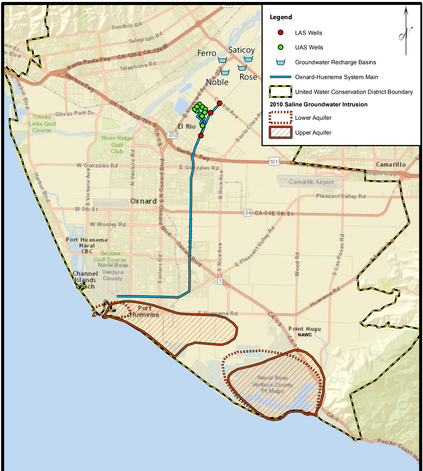
Figure 6-3 Saline Groundwater Intrusion Oxnard Plain Basin
