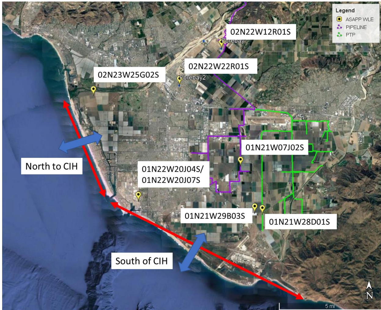
Figure 4.9. Locations for comparing groundwater levels and seawater intrusion for ASAPP scenarios. Well locations are indicated by yellow symbols and State Well Number. Seawater intrusion is calculated separately for the Oxnard Plain coastal zone north and south of the Channel Islands Harbor (CIH) entrance. Approximate extent of each zone is indicated by the red arrows.
