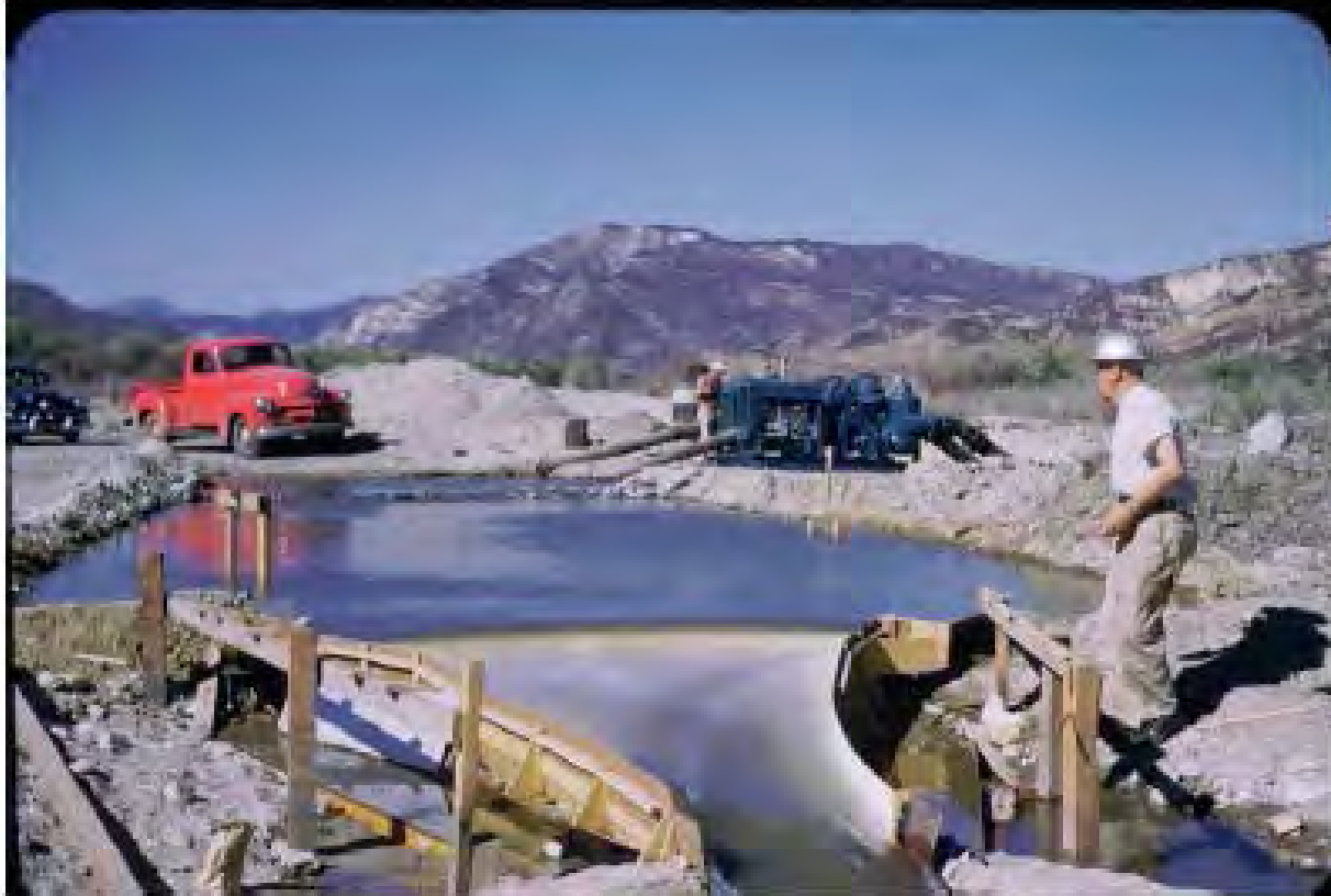
Figure 2-8 Spillway Scale Model Testing
