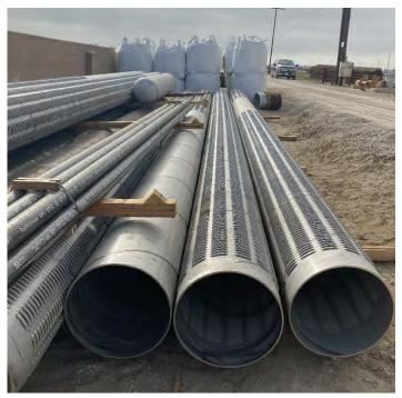
Figure 2 – OH Well Replacement Project – Well Casing Prior to Installation
