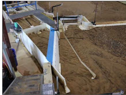
Sediment deposit after test DD-2 (6,000 cfs river, 1,500 cfs diversion)
