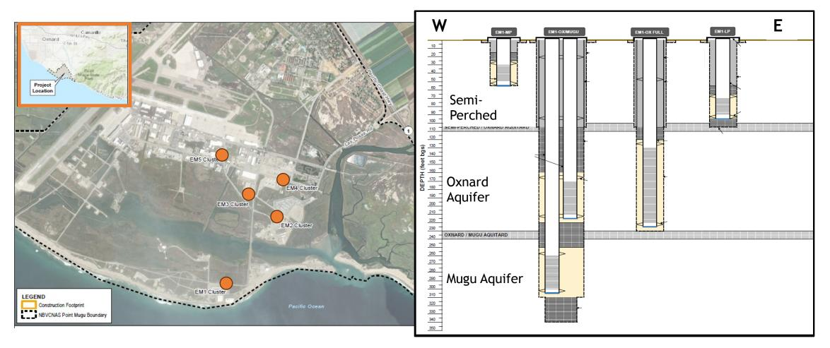
New Monitoring Wells will be used to collect date that help accelerates project design and permitting
