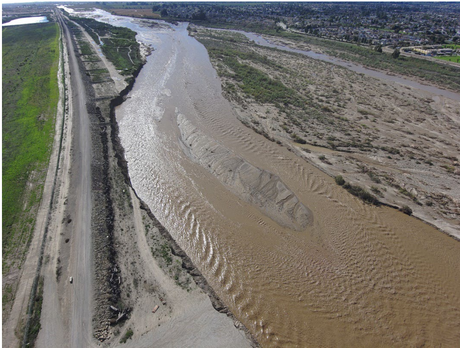
Figure 2 – Erosion of Santa Clara River Levee adjacent to Ferro Basin
